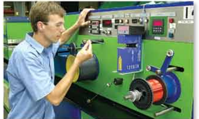
Continuous in-line diameter measurement provides effective quality assurance on high speed enameling lines. The data can be converted into reports that record the minimum, maximum and average dimensions, and the process capability for a given production run.
