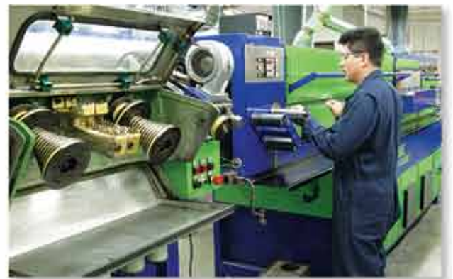
In-line drawing machines can be utilized on any enameling oven, enabling production efficiencies as well as excellent bare wire quality.
