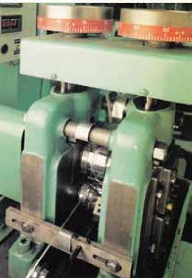
Reusch Model#154 Rolling mill provides state-of-the-art capabilities for production of tight tolerance flat conductors. Sizes range from .0005" thickness to 2" widths with tolerances as close as +.00015".
