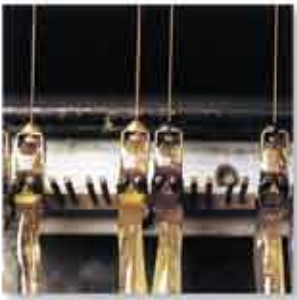
Metering dies are used to apply smooth, concentric film coats to wires sizes AWG 30 and heavier.
