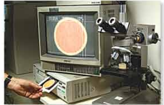
The Olympus Stereo Microscope, together with the Boeckeler Measurement and Sony Imaging System, can take cross-sectional measurements as small as 3 microns. Measurements include X-axis / Y-axis measurements as well as corner radius. Verification can then be sent to our customers by either a printed color photograph or digital image sent via e-mail.
