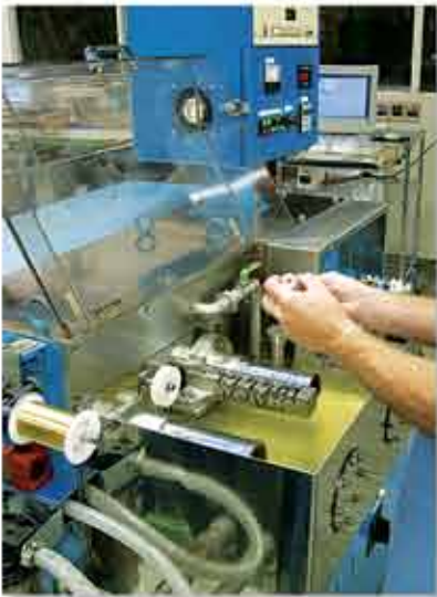
This specially designed machine draws precious metals to ultra-fine sizes in standard and custom diameters and tempers.
