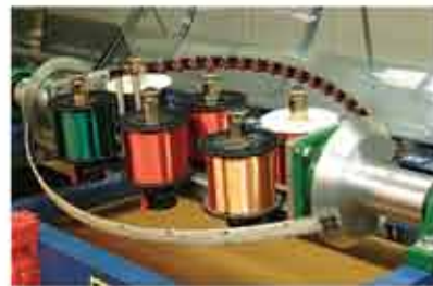
Twistite™ magnet wire, up to 50 twists per inch, is produced for numerous electronic applications, utilizing a wide range of conductor materials, insulations and colors.
