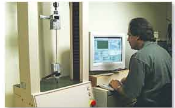
The Satec Model T1000, incorporated with Satec's "Partner" software, provides precise values for the physical and mechanical properties of metals. Specific tensile strength, break load (from 2 grams to 1,000 pounds), yield strength, elongation and bond strength data is obtained on a wide range of bare and insulated wire and ribbon. Reports can be generated and sent to our customers for test value verification.
